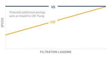
Variable Speed: RPM set high to maintain minimum flow Variable Speed and Flow:
