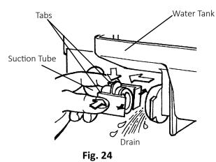
Reconnect the suction tube as illustrated. See Fig. 25. Make sure the tabs lock into place; a loose fitting may cause a water leak.
