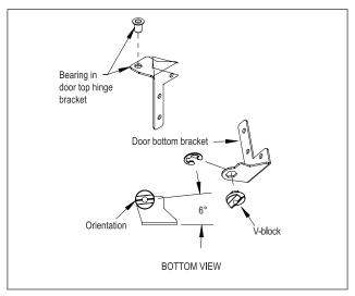
Figure 13. Bearing and V-Block
