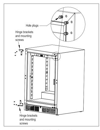
Figure 8. Hinge Removal
