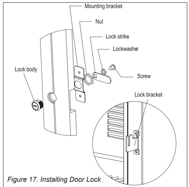
Figure 17. Installing Door Lock
