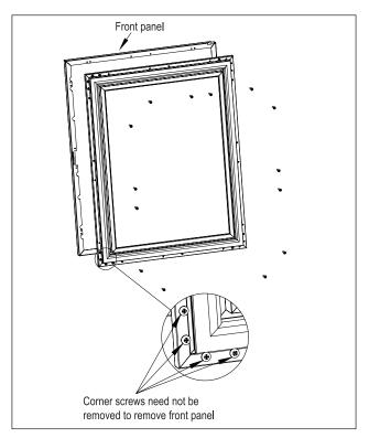
Figure 11. Removing Front Panel
