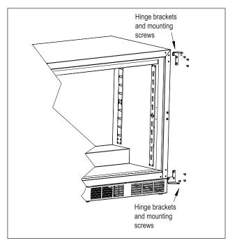
Figure 9. Hinge Installation
