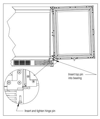
Figure 16. Installing Door
