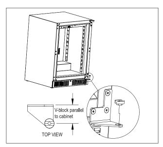
Figure 15. Installing V-Block
