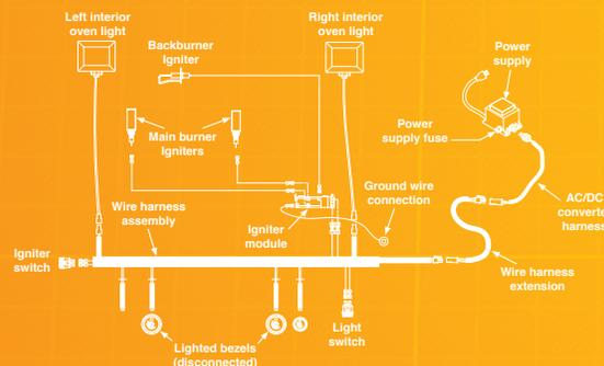
\* 24" model shown. Model wire vary between models, a wire diagram specific to each unit can be found affixed to the inside of the control panel.
