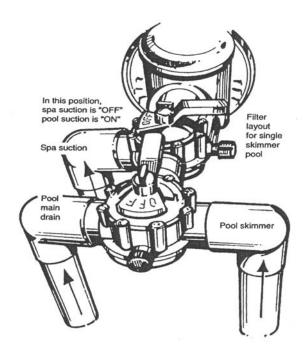
This plumbing illustration is an example of a one skimmer and main drain pool set-up with the spa suction valve in front of the pump. In this position the spa suction is closed and the pool is operational
