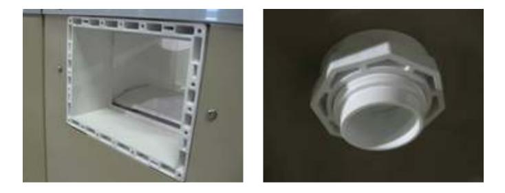
To install the return fitting, you need to un-thread the retaining nut from the fitting. Insert the threads through the pre-punched hole from the inside of the pool and tighten the retaining nut to the back of the fitting. **Be careful not over tighten this nut**.
