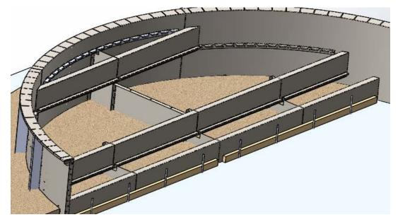
Once the concrete base is hardened add #57 gravel (or other noncompressible backfill) up to within 4"  $\pm$  of each tread.
