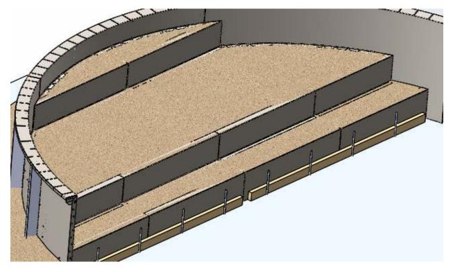
When the concrete is hardened peel off the tape that was placed on the top side of the liner track and make sure everything is smooth.
