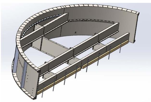
At this point it is best to tape the top and bottom of the liner track to prevent fines or concrete from entering the gap.
