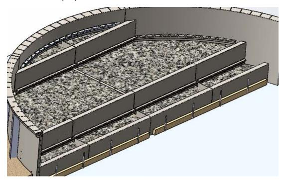
Pour 4" of concrete on each level tread. Screed it off level with the liner tracks and top of treads.
