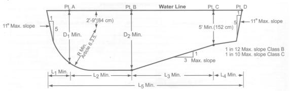
NOTE: L4 is a minimum dimension to allow sufficient length opposite the board. This may of course be lengthened to form the shallow portion of the pool. L2, L3, L4 combined represent the minimum distance from the tip of board to pool wall opposite diving equipment.
