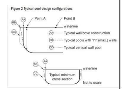
5.2 Perimeter shape. No limits are specified for shapes of pools. Consideration shall be given to circulation and safety to the user.
