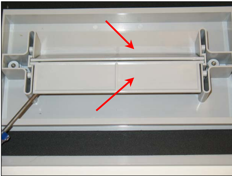
Inlet flaps, check for free movement.
