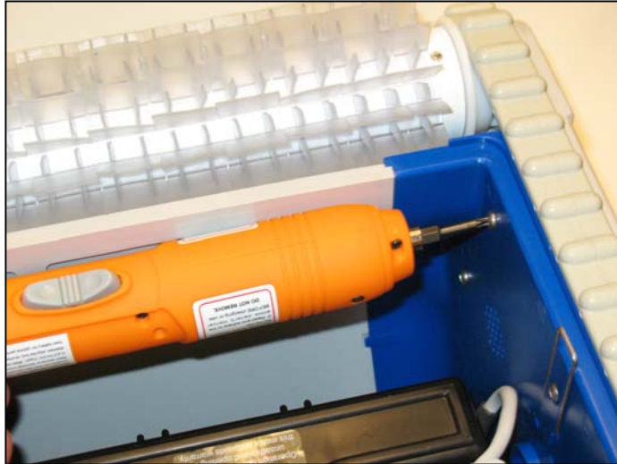
Screw removal, opposite side cover, non-drive side.
