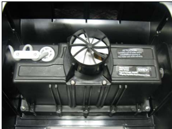
Filter cartridge removed
