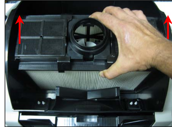
Lift to remove Filter Bucket Housing
