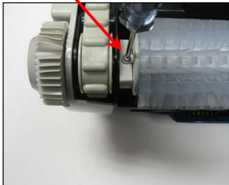
Unscrew T20 screws from each side of roller.
