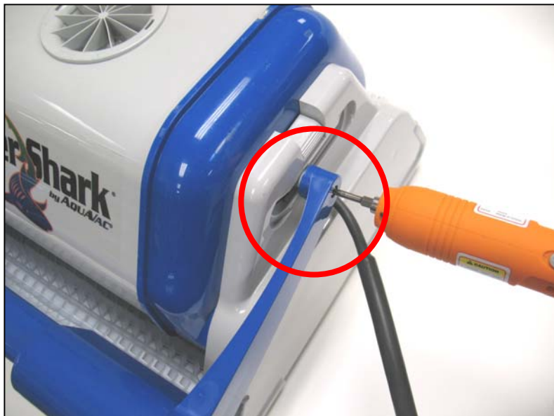
Handle removal 1 screw each end
