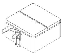
**C)** Ensure that the Premium Cover Lift is deployed, as shown.
