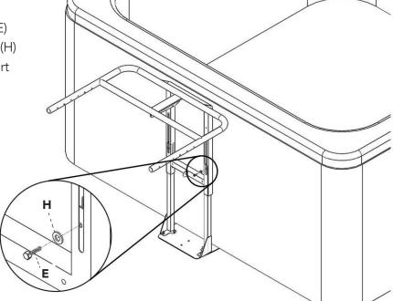
NOTE: Steps 5 and 6 are used only if using a side mount setup and NOT using the Base Plate (FF).
