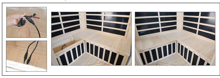
8. Lift the ROOF above the sauna, feeding the heater cables on side & back walls, and the wire harnesses and power plug in back left corner, through the corresponding holes on perimeter of roof.
