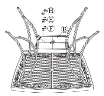
After making any necessary adjustments to the alignment of the table, use the hex bolt driver and hex wrench to tighten all bolts . **Note:** each bolt must be tightened a few revolutions at a time. In order to apply equal pressure to all bolt joints, we recommend working in a cross corner (X fashion). Repeat until all bolts are tight. **Do not over tighten.** Over tightening may strip bolts. Cover all bolts with covers.
