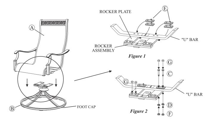
Tighten all nuts and bolts with the hex wrenches provided. **Ensure the bolts are FULLY tightened.** Remove arrow labels from "U" bar and rocker assembly. Cover bolts with bolt covers.
