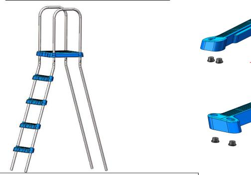
① Lay the platform, inner ladder, and outside handrail on the ground. Follow the above illustration to connect handrails. Refer to **ASSEMBLY DETAIL C** for screw and washer order. After this step, the ladder should be in an "A" shape, as shown.
