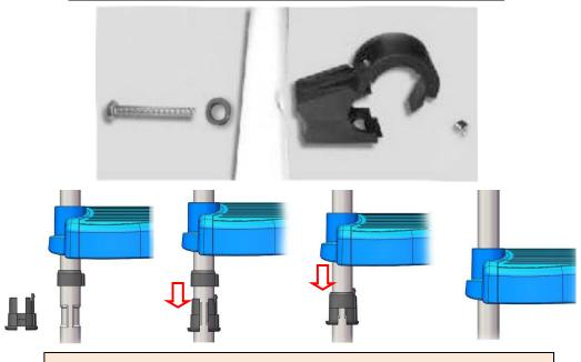
ASSEMBLY DETAIL A - Detail Diagrams of Step/Platform installation
