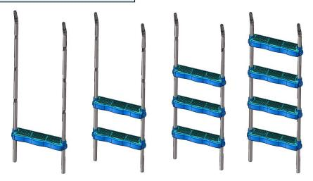
Follow <u>ASSEMBLY DETAIL A</u> to install the first step through the fourth step of inner ladder. Note: The end with the White Plug should face UPWARD.
