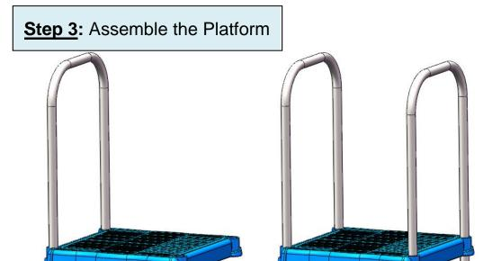
Follow ASSEMBLY DETAIL A to install the platform to the connection bridge.
