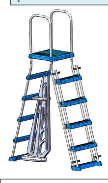
① Insert the removable Safety Steps into the holes in the Bottom Outside Step. Tilt the Removable Safety Steps up, aligned with the Outside Rails.
