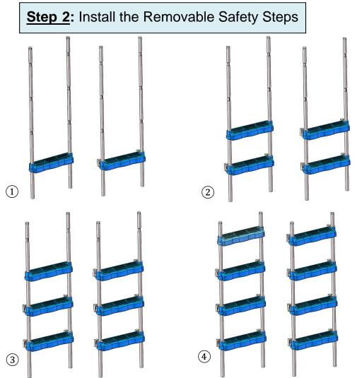
Follow <u>ASSEMBLY DETAIL A</u> to install the Steps and then Follow <u>ASSEMBLY DETAIL B</u> to install two bushings on as shown in sub-steps ① through ④, above. For easier installation, remove the White Plugs first and when the bushings are installed, re-install the white plug.
