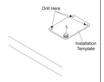
**12.** Secure the Base (1) to the deck using the four 3/8" Bolts (5), Stainless Steel Washers (6), and Rubber Washers (7).
