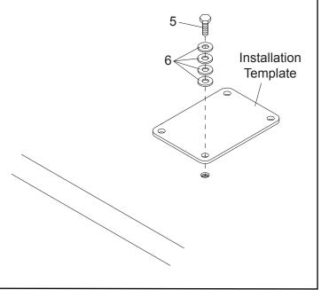
**10.** With the Installation Template tightly secured to the pool deck, drill the remaining three holes to a depth of 1 5/8". **Note:** Remember to account for the thickness of the Installation Template.
