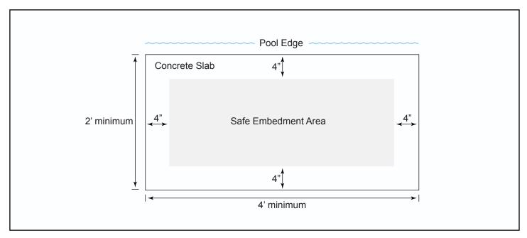
FIGURE 1: CONCRETE SLAB REQUIREMENTS
