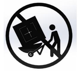
DO NOT USE A WHEELBARROW OR OTHER UNBALANCED EQUIPMENT TO MOVE UNIT
