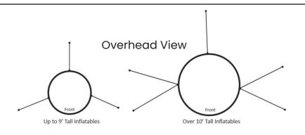
To properly secure your inflatable, install the upper tie downs according to the above graphic. Note that two of the side tie downs must angle forward by at least 30 degrees. Adjust stakes as needed to assure that the inflatable is fully upright and positioned correctly. When the inflatable is correctly positioned and all stakes have been placed, push all of the stakes fully into the ground.
