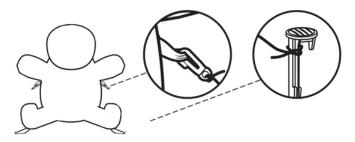
For inflatables under 9-feet tall, install at least three upper tie downs. For inflatables over 10-feet tall, you will need to install four or more upper tie downs, depending on the inflatable.
