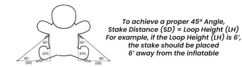
The angle of the rope to the ground should be 45 degrees (see diagram above). To achieve a 45-degree angle, the stake distance (SD) from the inflatable should be roughly equal to the loop height (LH) on the inflatable.
