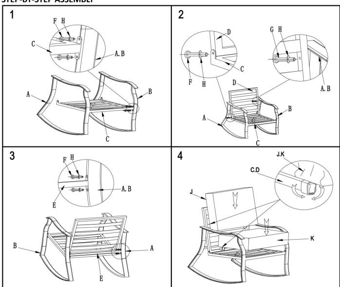
Tighten all the bolts using Allen Key (I). Repeat the steps for second chair.
