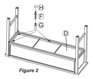
Attach the bottom shelf to two table legs by using four 1/4"x35 mm bolts and washers as shown in *Figure 3*. Guide the bolts through the holes in the bottom shelf, into the pre-drilled holes in the table legs. **Hand tighten 2-3 turns only.**
