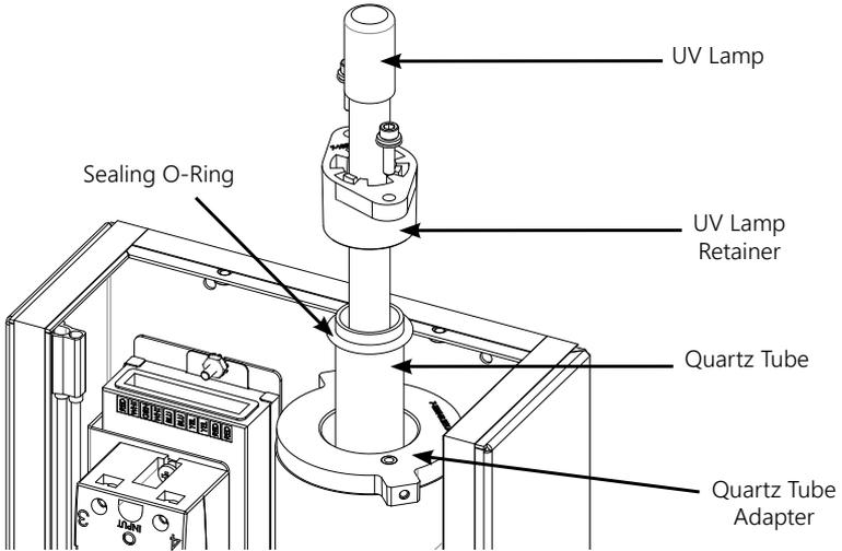
**Figure 6: Lamp and Quartz Tube Removal**
