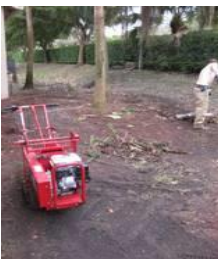
Sod Cutter Removal
